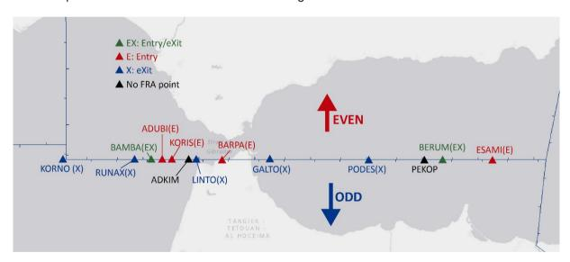
FRA Horizontal Entry Point (E) is a published Significant Point on the horizontal boundary of the Free Route Airspace from which FRA operations are permitted while an Exit Point (X) is a Point to which FRA operations are permitted.
